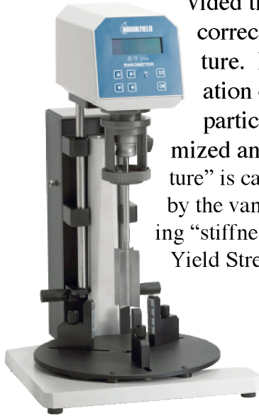
Figure 4 Brookfield R/S-SST Rheometer with Vane Spindle Keeps Particulate Additives in Suspension during Viscosity Measurement
