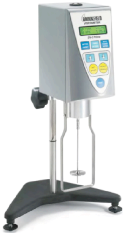
Figure 1: Standard Benchtop Rotational Viscometer
