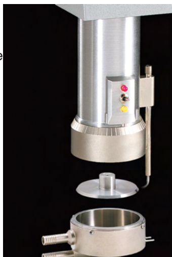
Figure 2 / Sample Cup Spindle for Wells/Brookfield Cone/Plate Instrument. Sample Goes On Plate Inside Cup. Ports On Cup Connect To Circulating Temperature Bath.
