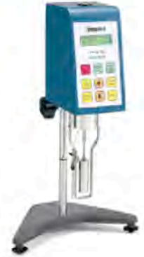
Figure 2: Brookfield DV-II+Pro Viscometer with automatic test capability
