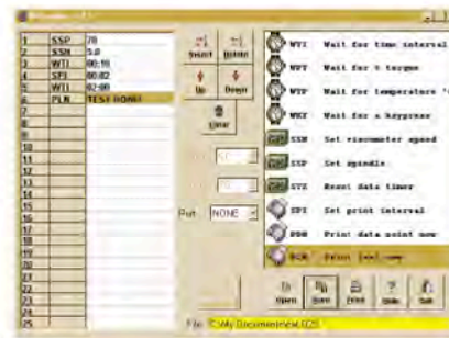
Figure 3: DV Loader Software allows QC to create detailed tests which run automatically
