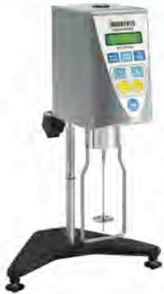
Figure 1: Brookfield DV-I Prime Viscometer with RV-4 Spindle
