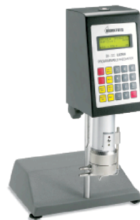
Figure 3: Brookfield Cone/Plate Rheometer for Evaluating Viscosity Behavior of Medicinal Mixtures
