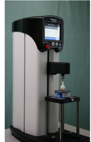
Figure 1 CTX Texture Analyzer with 25.4 mm dia. Spherical Probe (TA43)
