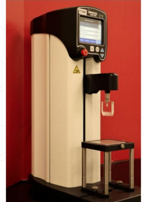
Figure 1 Brookfield CTX Texture Analyzer fitted with 10kg loadcell & acrylic knife blade
