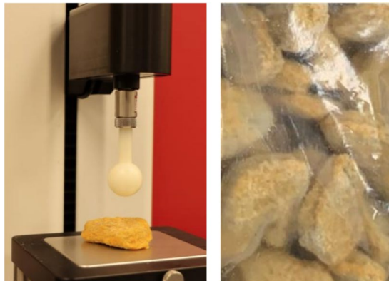
Figure 3 25.4mm \phi ball probe (TA43) for testing Flat Sample
