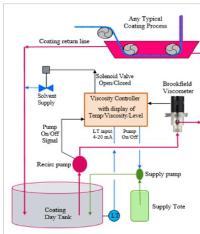
Figure 1: Typical Viscosity Automatic Control System
