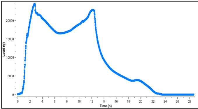
Figure 3: Force vs. time to deform a packaging container over a specified distance of 40 mm.
