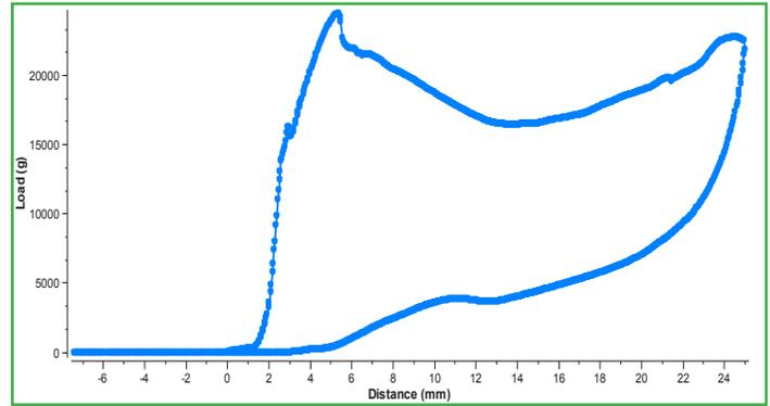
Figure 4: Force vs. distance for the deformation of the same packaging container.
