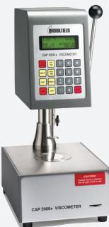
Viscometer Specific for Paints and Coatings
