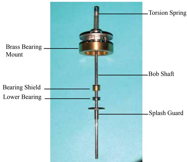
17. Slide the bob shaft up through the upper brass bearing mount. Turn the bob shaft in the direction that allows the “Flat” located at the top of the bob shaft to be positioned towards you.
