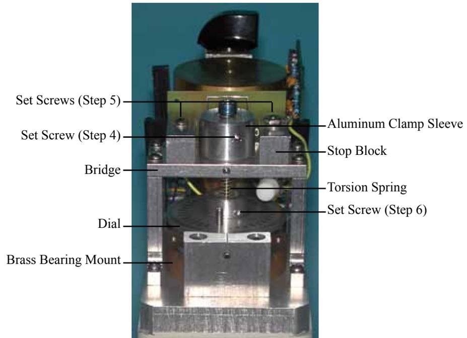
8. Remove the four screws from the bridge and lay it gently to the right side.
