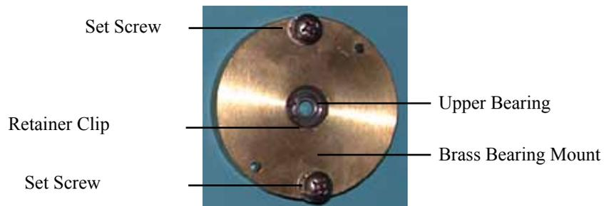
11. The upper bearing is located inside the brass bearing mount. Use the retainer ring pliers to remove the retainer ring. Push the bearing upwards to remove the upper bearing from the brass bearing mount.
