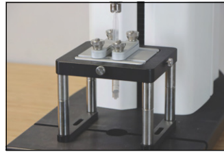
Syringe Test Fixture Measuring the force required to push or pull syringe plunger. Important to all syringe markets. Base Table required. TA-STJ P
