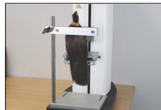
Hair Combability Fixture Measures the effect of hair dye, shampoos and conditioners on the compatibility of hair. TA-HCF C
