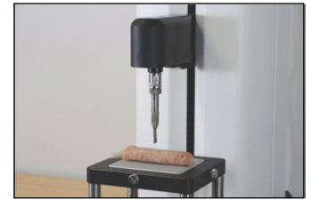
Shear Blade For cutting tests, especially meat, poultry, fish or similar products. Fixture or rotary base table recommended. TA-52 MOHRS F
