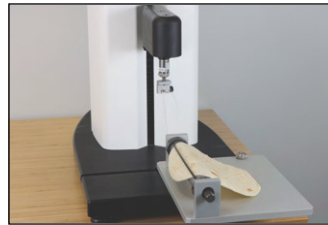
Tortilla Roll Up Fixture Evaluates changes in corn tortilla texture per AACC technical paper by measuring the force to roll up a tortilla. TA-TRF F
